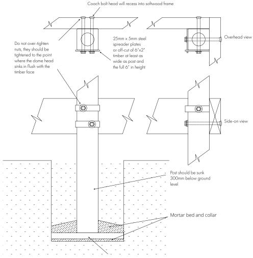
300 mm square slab or  $440 \text{mm} \times 215 \text{mm}$  breeze block base
