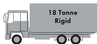
Lengths Max. 7m Max. Carrying Weight: 9.5 Tonnes*
