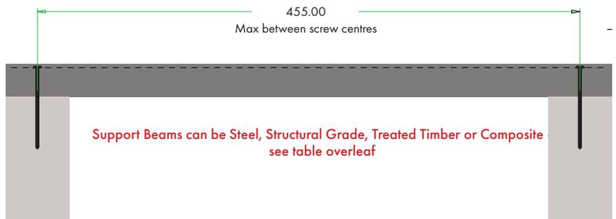
ECODEK® 'AT' 21MM GROOVED/RIBBED DECK BOARD STRENGTH CHARACTERISTICS, AND SPAN TABLE CAN BE FOUND ON OUR WEBSITE
