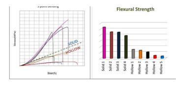
Ecodek only supply SOLID composite deck boards and concerns have recently been expressed to us from a variety of sources that some manufacturers' hollow composite boards are performing poorly and failing, sometimes within 12 months of use.
