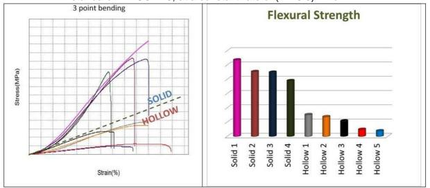
The results obtained from the compared samples are depicted in the figure above. There is a clear differentiation between the solid and hollow samples with regards to mechanical properties. The performance of the solid samples that we tested significantly exceeds that of the hollow samples, both in terms of elasticity and maximum strength.
